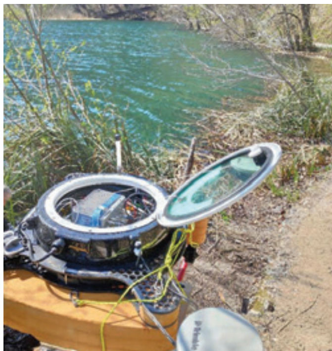
The PlaDyBath platform ready to begin bathymetric survey of the lakes.
