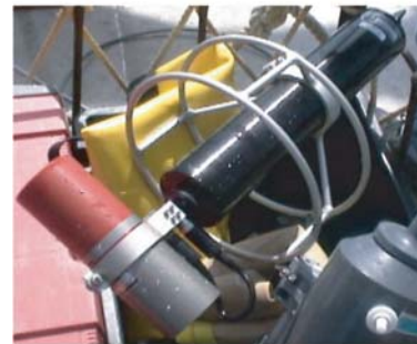
Fig. 7. Imagenex two axes SONAR system. The red section houses the pencil beam transducer, the grey section houses the electronics and motor for the 881A and the black case houses the azimuth rotation motor, control and overall electronics for the system.
