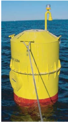
Fig. 5. Surface feed buoy platform for controlling the feeding operation, observing the fish in the cage below and telemetering the images to shore [2].
