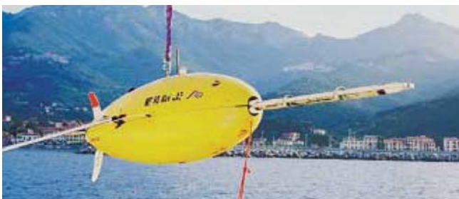
AUV used in GOATS project.
